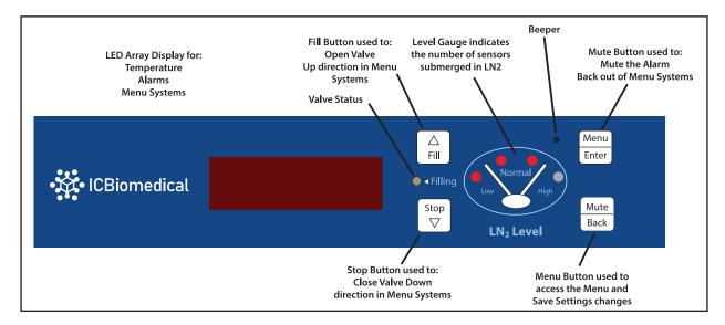
CS100 Control Systems - LS Series Cryostorage Systems
