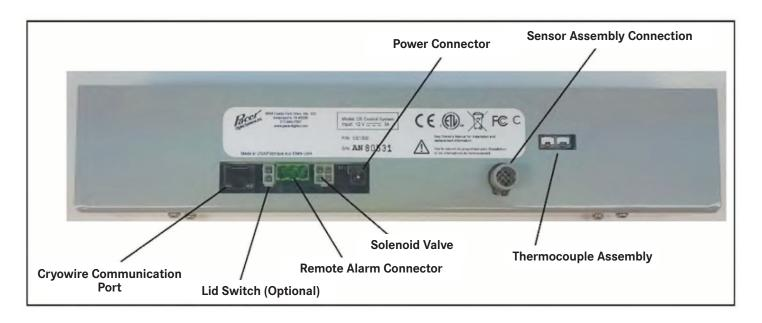
Connect the thermocouple plug of the harness assembly into the control at the thermocouple plug. This is located on the right edge of the control if looking at it from the front. One of the blades on the plug is slightly wider insuring that it is plugged in correctly. Copper blade should plug into copper colored plug. On the other end of the harness, connect the Thermocouple assembly into the plug insuring that copper colored blade is plugged into copper colored contact on receptacle.
