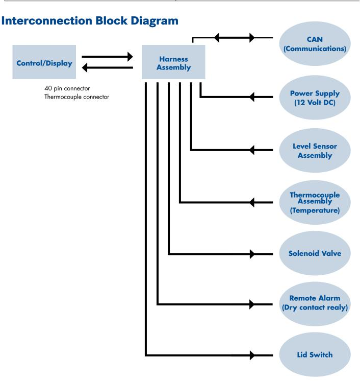
**CS100** Control Systems - LS Series Cryostorage Systems
