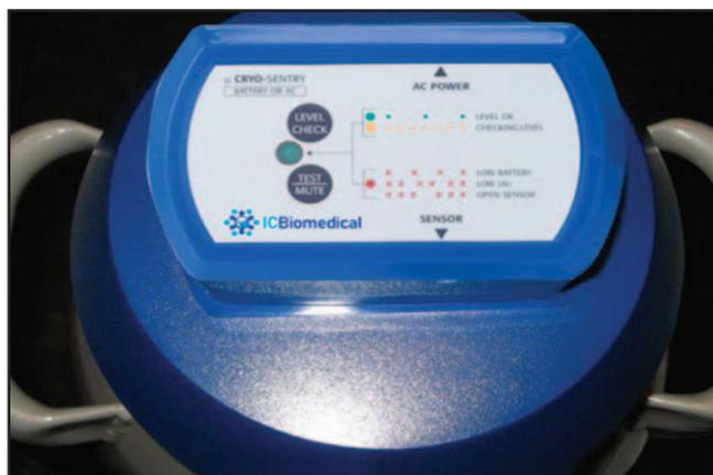
The Cryo-Sentry is an optional accessory for select IC Biomedical portable liquid nitrogen freezers. Cryo-Sentry provides visual and audible alarms when the liquid nitrogen level drops below a preset level – usually 25 percent of the container’s capacity.
